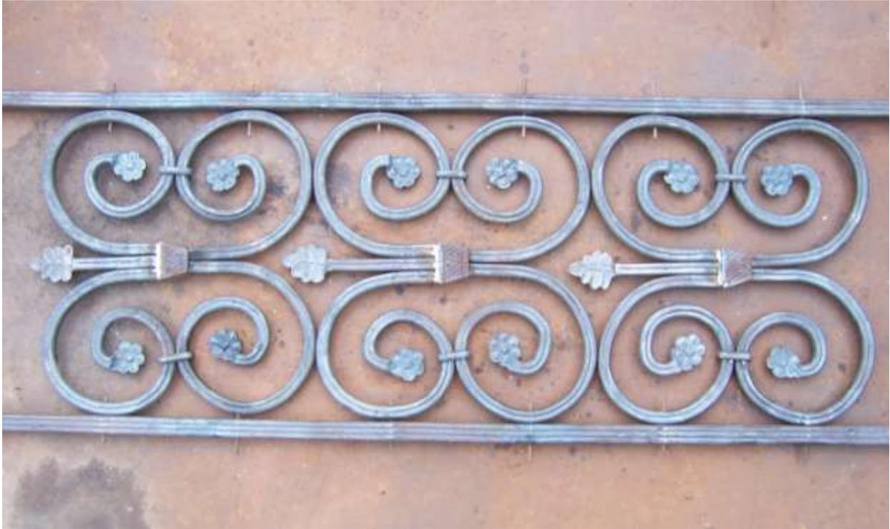
We will focus on early traditional European ironwork. The primary demo piece will be based on the 13<sup>th</sup> century French style, pictured. We will discuss making and using dies and swages with a power hammer or striker, traditional joinery techniques and assembly.
